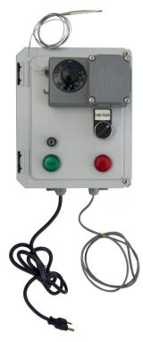
**PLAHBO Audible Power Loss Alarm:** The alarm consists of the cabinet, battery, battery charger, relays, 95-decible horn, six foot power cord and plug. The alarm is designed to activate the horn if the enclosure loses electrical power.
